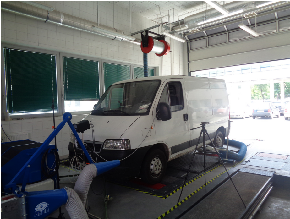
Fig. 5. Dyno test bench data recording, with OBD acquisition shown. The audio recorder is placed on the tripod
