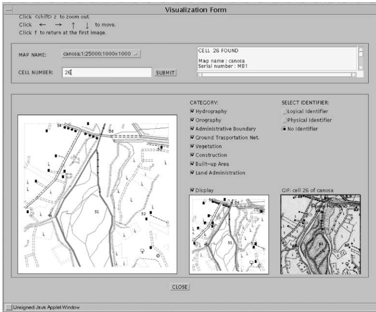
Fig. 2. INGENS graphical user interface displaying map data (upper left corner), cell data (upper right corner), zoomed area (left), geographical objects in the cell (middle), and original bitmap (right).
