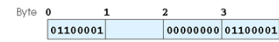
Fig. 10.1) A possible storage alignment for a variable of type struct example showing an undefined area in memory.
