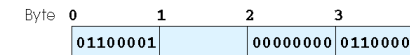
Fig. 10.1) A possible storage alignment for a variable of type struct example showing an undefined area in memory.
