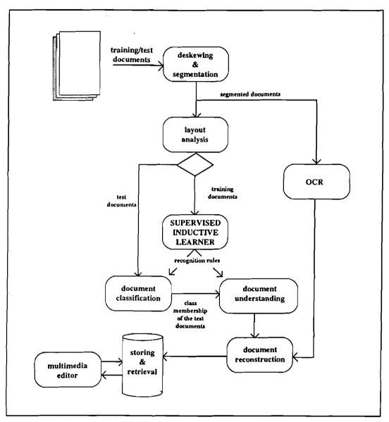
Figure 3. Architecture of PLRS. After having scanned a document, the system detects a possible skew in the document image and corrects it by means of a rotation. Then the document image is segmented into blocks, which are grouped together by the layout analysis. The supervised inductive learner produces rules useful for both document classification and document understanding. Finally, the document is reconstructed by exploiting information read by the OCR.
