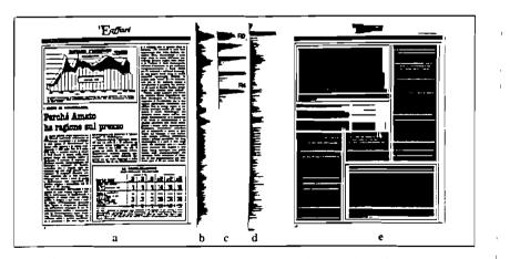
**Figure 4.** (a) Scanned document, (b) horizontal histogram, (c) sample region R0 and its successive rotations R1, R2, R3, R4, where the last three determine the points of the interpolation, (d) the horizontal histogram after the rotation, (e) result of the smoothing process.
