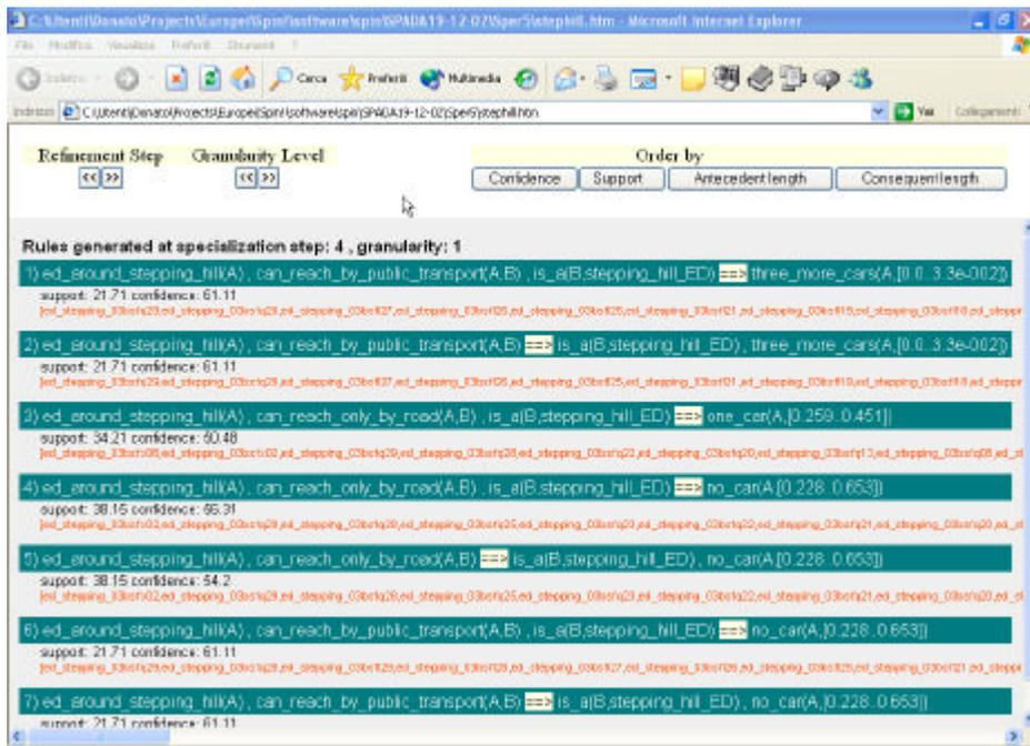
Figure 5. Browsing results of the SPADA system. The user can select the refinement (or specialization) step and the granularity level. Rules are reported in the order in which they are generated, but they can be sorted in a decreasing order by confidence, support, antecedent length and consequent length. In addition to usual confidence and support values, the name of the reference EDs supporting the rule is shown. Results can be easily shown on a map.
