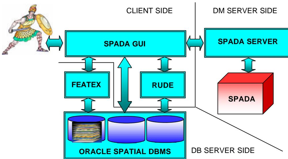
Figure 1. The software architecture of ARES
