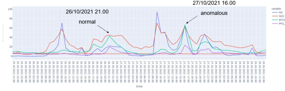
**Fig. 6.** Concentrations per hour of NO, NO<sub>2</sub>, PM10 and PM2.5 pollutants during October 2021, from Loallmenningen station.
