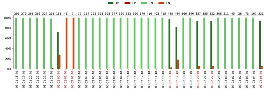
**Fig. 11.** Hour-by-hour histograms indicating True positives, True negatives, False positives and False negatives for the first day of data.
