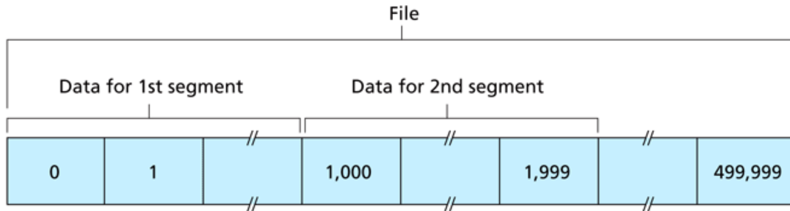
Figure 3.30 ♦ Dividing file data into TCP segments
